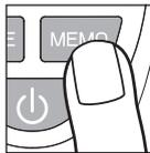
To clear the memory of previous temperatures, press and hold the “MEMO” button for 4 seconds.
